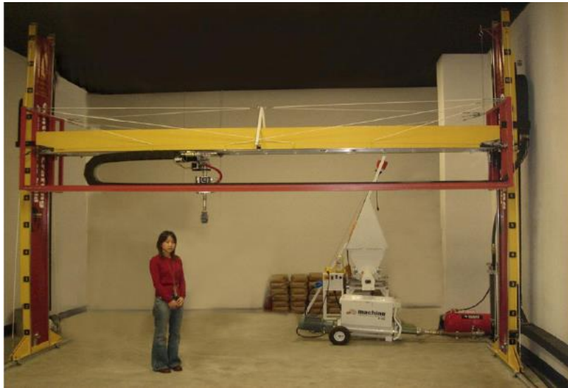
Figure 20: Contour Crafting single-nozzle gantry fabricator (Zhang 2013)
