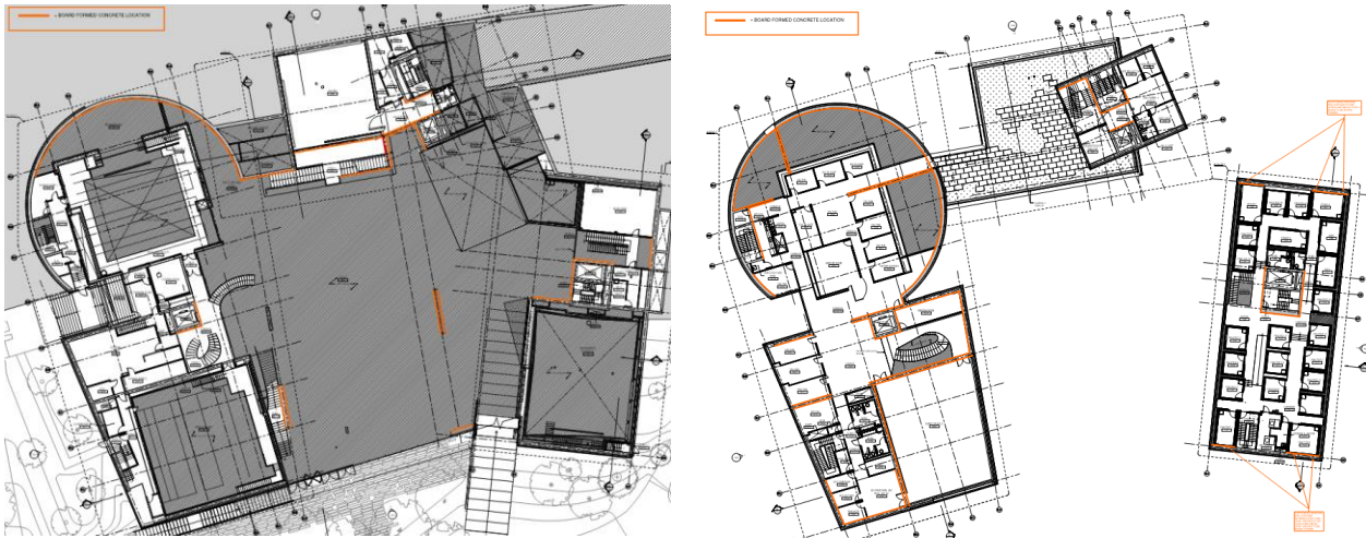
Figure 37: Board formed concrete locations shown in orange. The Mezzanine Level is shown on the left and Level 3 is shown on the right.
