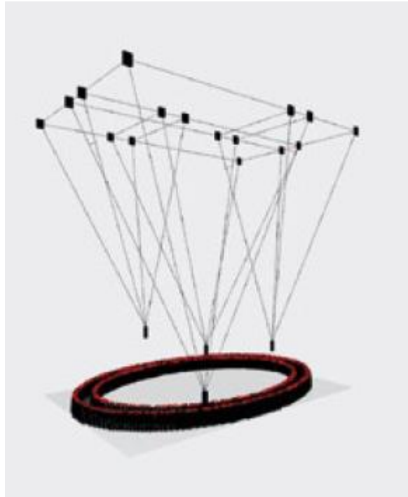
Figure 12: CableBot multi-node fabrication system designed for communicativeness (Oxman 2014)
